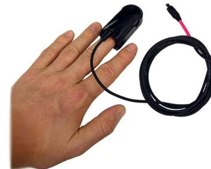
Figure 3. PPG monitoring system
