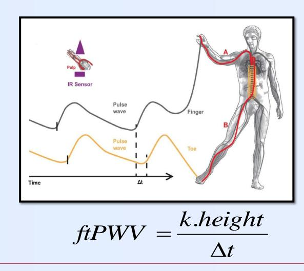
The pOpmètre ® has 2 photodiodes sensors, positioned on the finger and on the toe, next to the pulp artery. A particular attention was drawn on positioning of the toe sensor so that the pulp was in contact with the photodiode. Different signal processing was applied and no cut-off value was used for pulse height.
